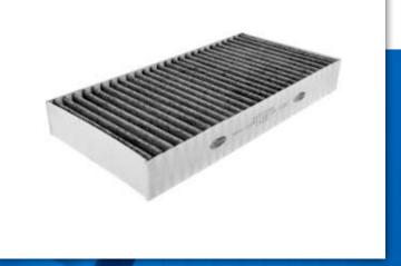
Alongside a range of cabin filters Comline also offers activated carbon options which offer an added layer of protection. The design of a carbon filter sees the media impregnated with activated carbon molecules that filter out harmful, ultra-fine gas particles such as Benzine or Ozone, plus absorb unpleasant odours which may otherwise enter the vehicle cabin.
