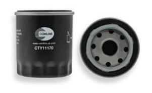
The **spin-on oil filter** takes its name from the process used to fit this type of part, where the entire filter, including housing, is quite literally 'spun on' to the vehicle's oil system. Spin-on filters are self-contained within a metal canister meaning the filter media, bypass and anti-drain valve, element cover and gasket are all built into the design.
