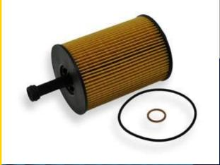
**Ecological (Eco)** oil filters, sometimes known as element or cartridge filters, differ from spinon variants as they are essentially a replacement of the filter element only. When replaced, the technician need only remove the existing filter element from the housing built into the design of the vehicle and replace with the fresh Eco filter.
