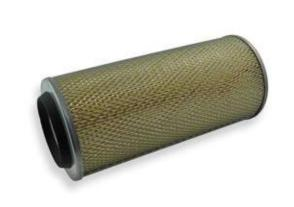
Visually a metal filter can look the same as a PU or PP variant, the crucial difference is that structural support is provided by a **metal**, **typically steel**, **frame** as opposed to moulded plastic. Such filters are mainly used within the Japanese and Korean vehicle parc.
